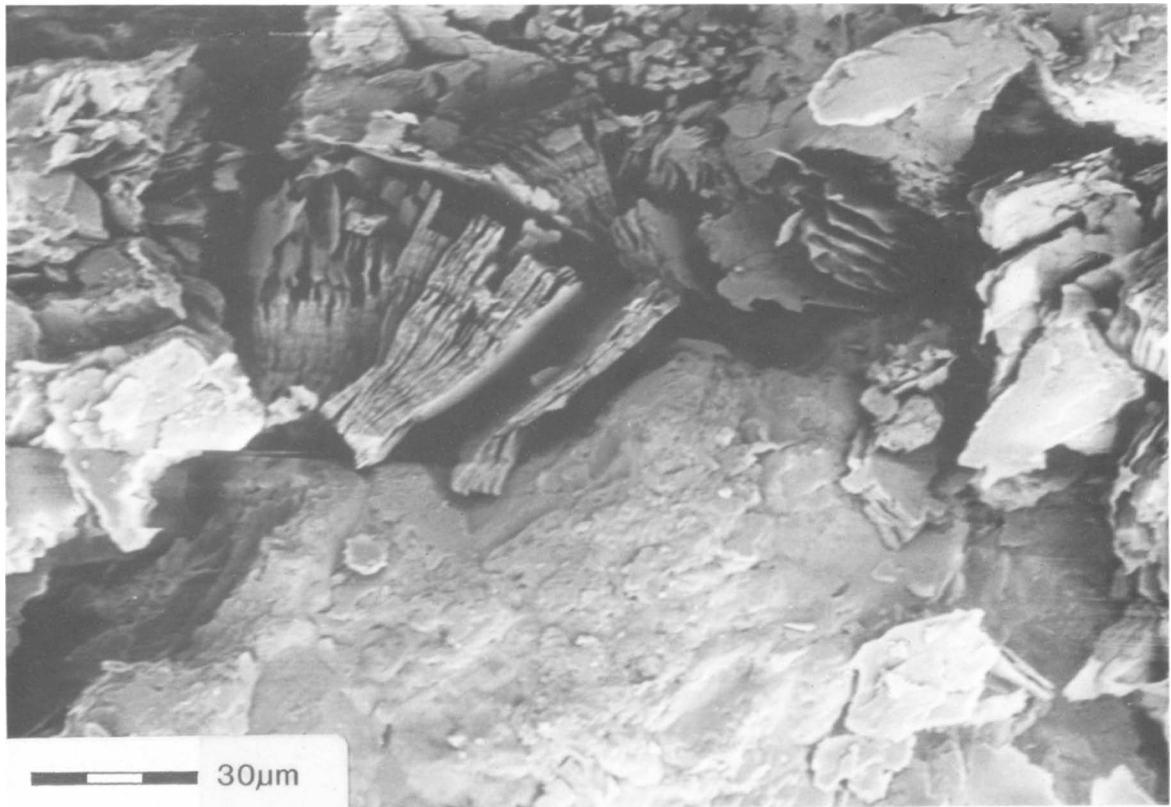
FIG. 9. Scanning electron microscope image (at magnification \times 900 ) of sandstone from the Mansfield Road sand mines. Books of authigenic kaolinite have grown in the pore space between quartz grains and now constitute the only cementing material.
